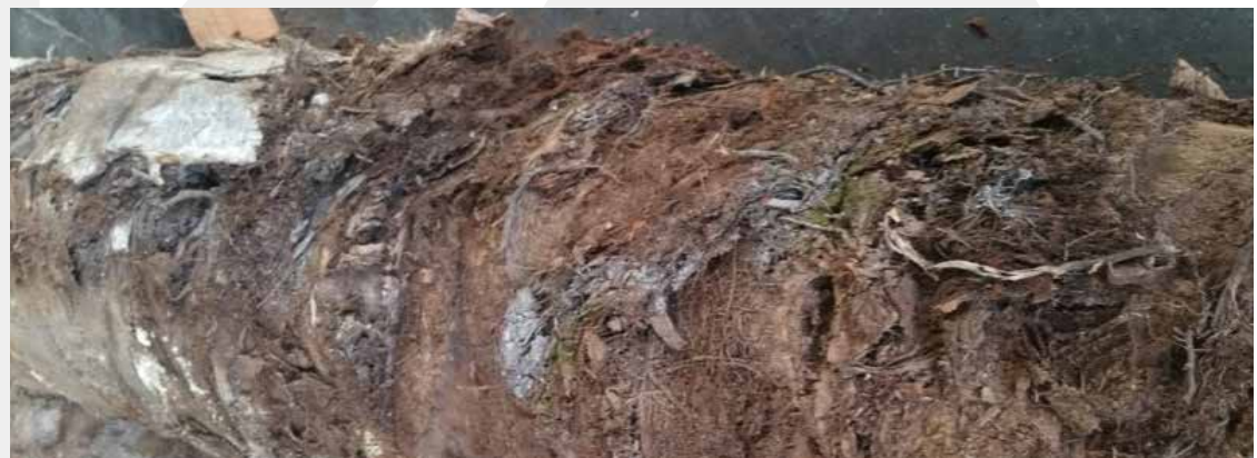
There are many impurities in the bark due to foreign substances and it will produce low quality pellets.
